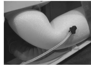
Defrost Sensor cable location
